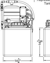
Note: Repressurization Pump/ Buffer Tank Stand Assembly can be removed from top of tank and placed on floor or shelf in close proximity of the tank. Use Remote Kit PN: 164-89116.
